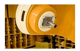
Circular fields generated by a Varian accelerator 2100C with conical collimators.
