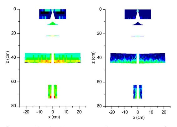
Left: map for high energy photons pointed to the phantom. Right: High energy electrons. Brighter colors correspond to higher importance.
